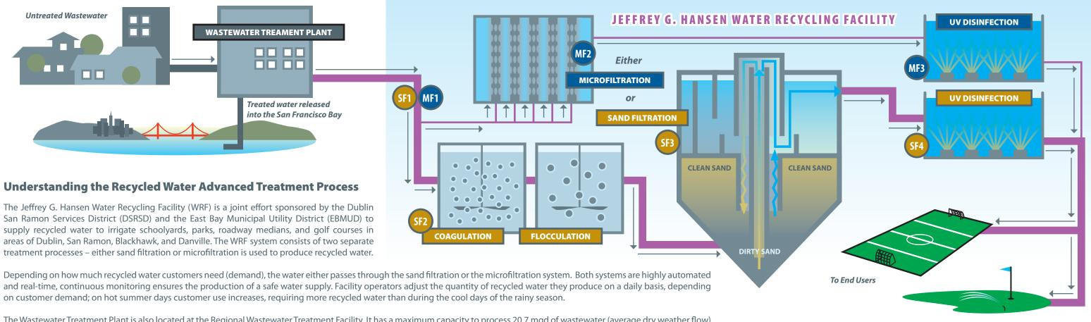
Depending on how much recycled water customers need (demand), the water either passes through the sand filtration or the microfiltration system. Both systems are highly automated and real-time, continuous monitoring ensures the production of a safe water supply. Facility operators adjust the quantity of recycled water they produce on a daily basis, depending
